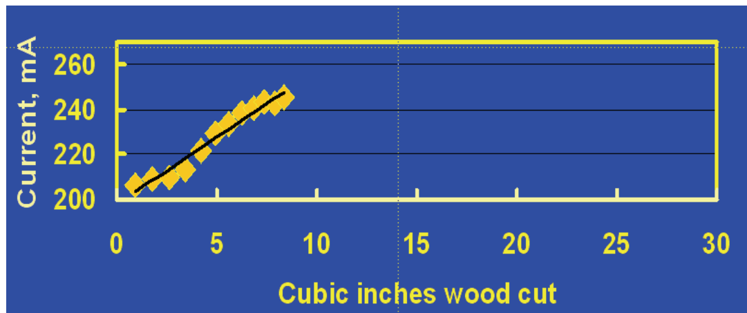
Figure 5. M2 blades began to wear immediately as indicated by increase in current to keep blade entering the wood at a constant rate. Cryotreated M2 behaved similarly. The students reported that both M2 and cryotreated M2 blades caused the wood to smoke during the final cuts on the 3 rd disc.
