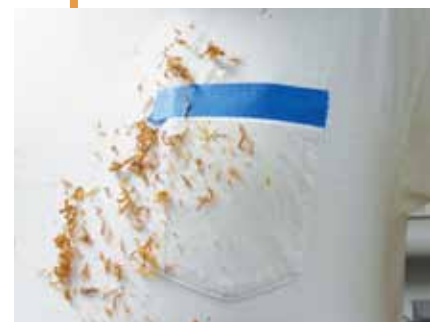
Taping your pocket closed prevents it from filling up with shavings. This is true for pant pockets, too.
