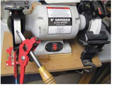
For everyday sharpening, many woodturners rely on a slow-speed grinder with two 8" × 1" white aluminum oxide wheels. On Jim Echter's machine, the left wheel has a TruGrind jig for sharpening gouges, skews, and parting tools. The right has a Veritas adjustable-angle platform for sharpening scrapers.
