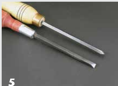
Skews come in different shank sizes and shapes. The square-shanked skews at right (aka, beading and parting tools) were fashioned from old screwdrivers.
