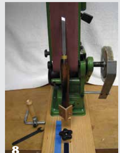
The author's shopmade belt sander sharpening station excels at forming flat bevels on skews.
