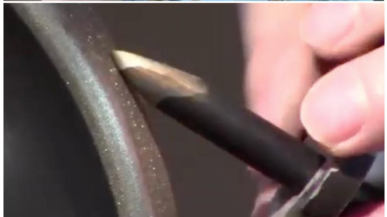
To the right is a double-beveled detail spindle gouge
