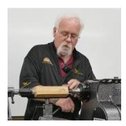
After getting the desired handle shape, bead the handle starting at the ferrule moving down. Using a beading tool lightly score lines to the base. Repeat beading process going deeper on the next pass, then finishing off the beads to full depth.
