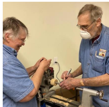
Kay & Bert Grant tapping a cup chuck for the 1" spindle
