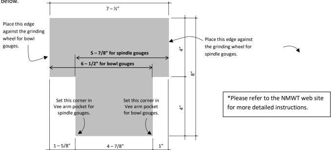
**Use of the Jig:** One edge of this set-up jig is used for spindle gouges, and the other edge for bowl gouges. Hold the edge of the jig for the tool to be sharpened vertically against the grinding wheel. Next, adjust the position of the Vee arm, so that the diagonally opposite bottom corner of this set-up jig is firmly held in the pocket of the Vee arm. Lock the Vee arm in this position. Care must be taken to hold the jig straight and true.
