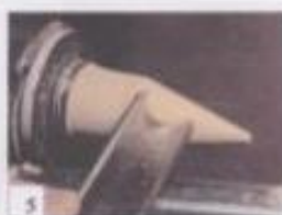
5 Use spindle roughing gouge to cut uniform 'cone' shape from mark on blank to a diameter of about 3/16" on right end of 'cone'.
