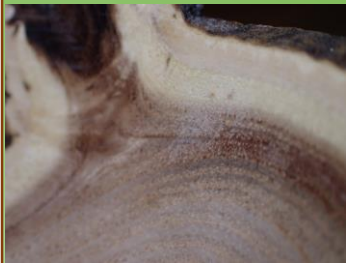
Pic: End-Grain Portion of Bowl Showing Minimal Tearout
