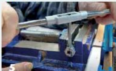
The author drills a hole and then taps threads for the cap screw, which will hold the blade in place during use.
