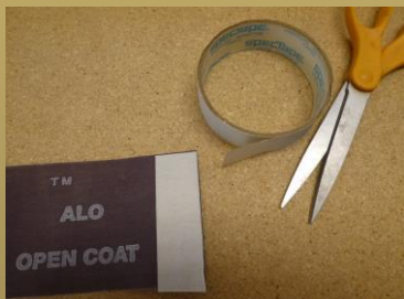
Photo 4: Two sided tape on back of sanding belt
