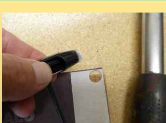
Photo 6: Removing disk from with hex wrench
