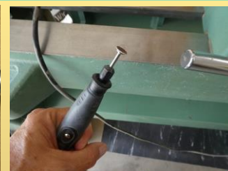
Photo 8: Disk on mandrel mounted in Dremel hand piece
