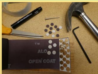
Photo 7: Seventeen disks from a 1.5" wide strip of tape on 3" sand paper belt
