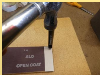
Photo 5: Striking punch with hammer
