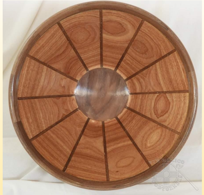
Second Stave Construction of bowl from a plank
