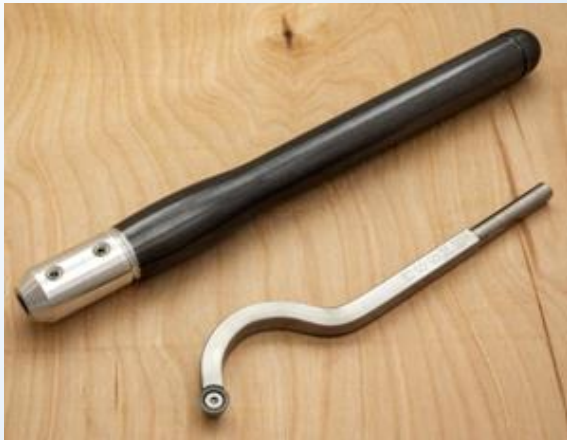
Typical "swan neck" hollowing tool for full size forms
