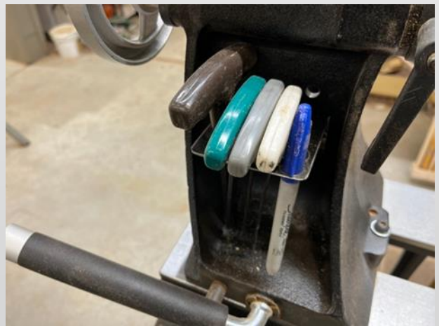
Added tool rack on outboard side of tailstock
