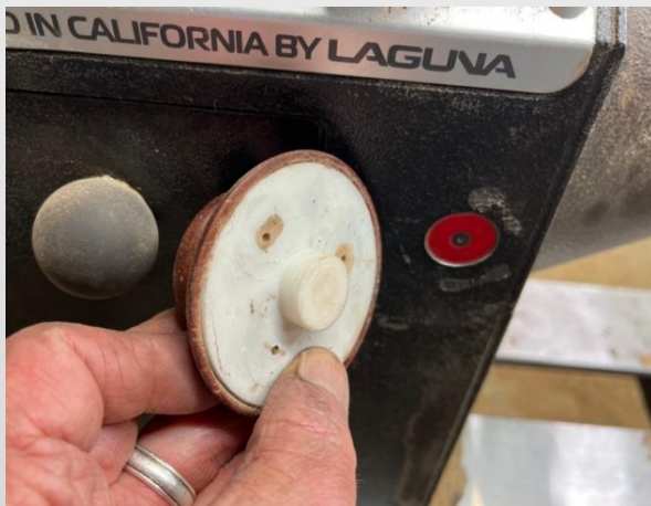
Puck with magnets and spindle lock button
