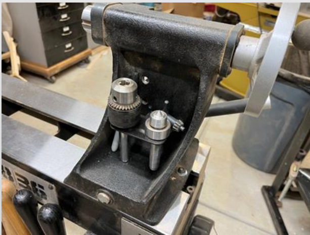
Tool rack on tailstock (came with lathe)
