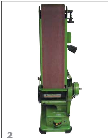
2 For this modification, unpack the parts but do not mount the disk sander or its table. Also, remove the back cover and bottom dust port, the sanding-belt guard, and the drive-belt cover.
