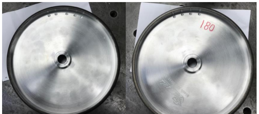
Figure 2 Photos showing drill holes on both sides of the same CBN wheel
