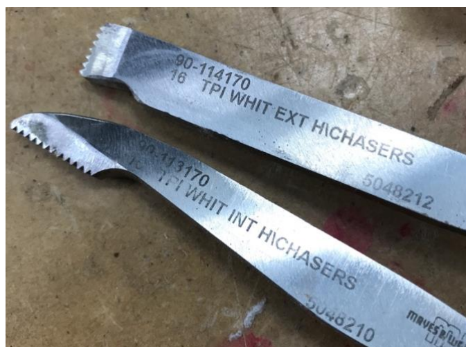
Above: 16 TPI thread chasing tools ground to optimize use.
